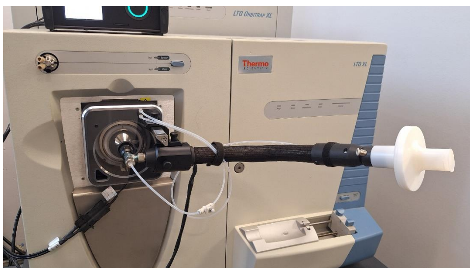
Figure 3: The SICRIT® Breath Analysis setup installed in diluted breath mode.
