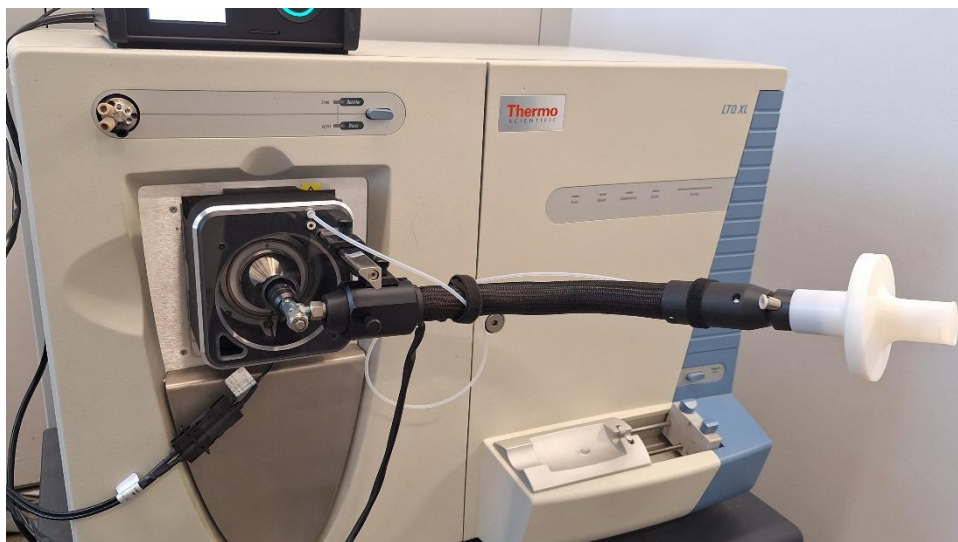
Figure 2: The SICRIT® Breath Analysis setup installed in non-diluted breath mode.
