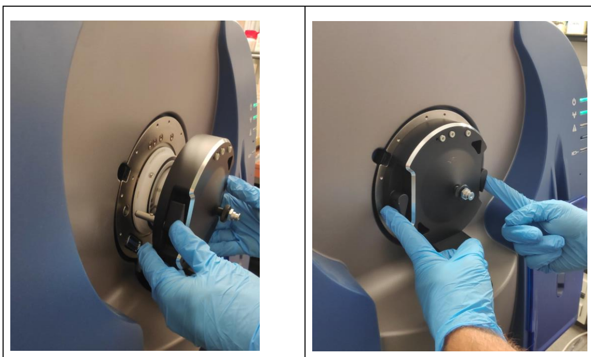
Figure 5: Installation of the SICRIT® MS Source housing onto the mount of the SCIEX MS-instrument.
