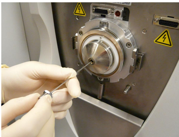
Figure 3: Installation of the SICRIT® Ion transfer capillary.
