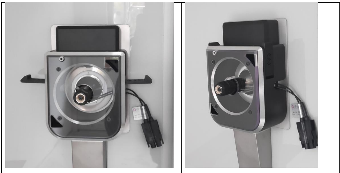
Figure 5: Installation of the SICRIT® NG retrofit housing to the mount of the MS-instrument by locking the levers.
