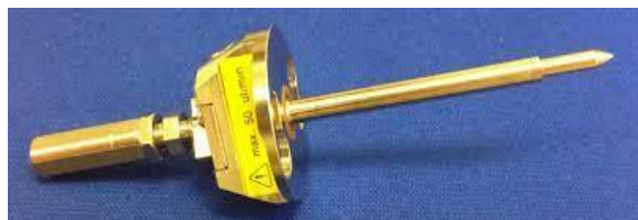
Figure 1: Different nebulizers options available for the LC/SFC module.
