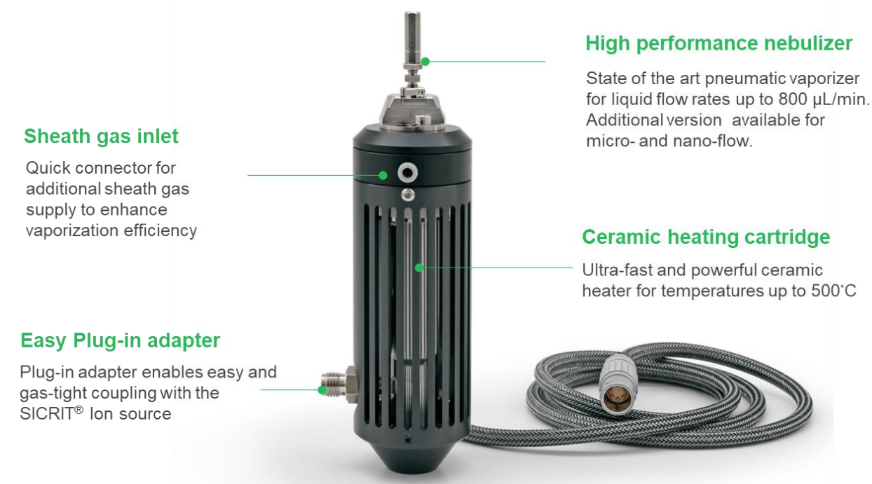
Figure 2: Components of the SICRIT ® LC/SFC Module.
