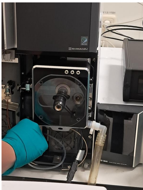
Figure 7: SICRIT® Interface SZ3 after complete installation.
