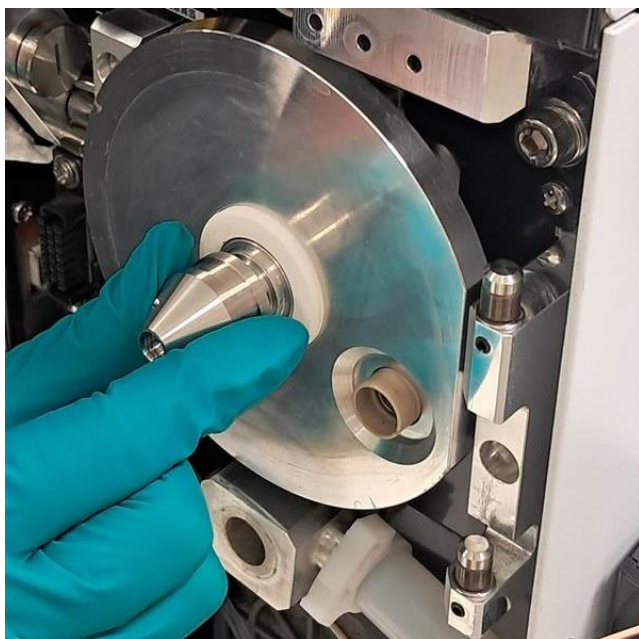
Figure 3: SICRIT® sample cone mounted onto the heat block.
